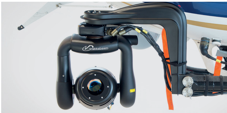
Airbus H135, Wescam MX-15 on camera bracket; Airbus H 135, Trakka A800 on Searchlight Bracket
