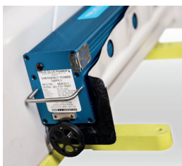
Battery for emergency retraction
