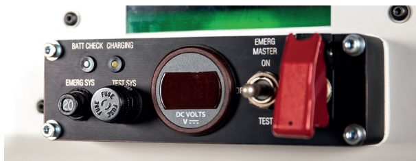
Control Panel for camera lift
